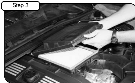
Unclip upper half of air box to remove lid and filter.
