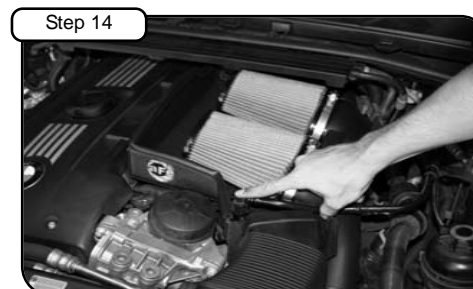
Install air filters and tighten with 5/16" nut driver and connect vacuum line.
