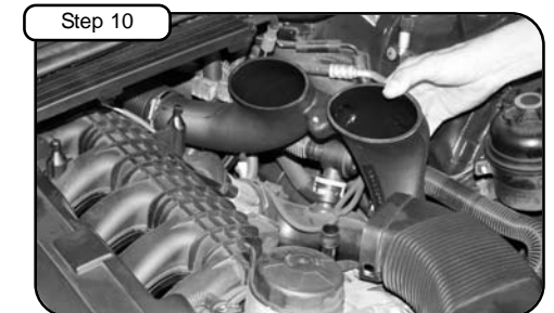
Install new tube into vehicle and pull back towards driver fender. Do not tighten clamps.
