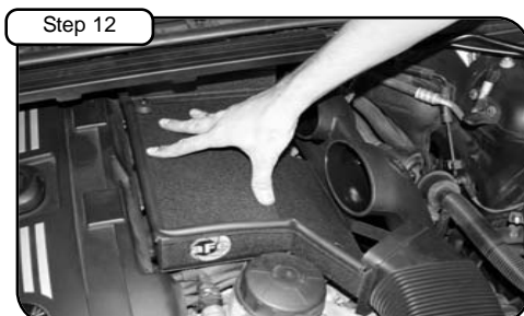
Push down housing allowing grommets to seat. Align threaded insert with hole on housing.
