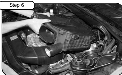
Remove complete air box from vehicle.
